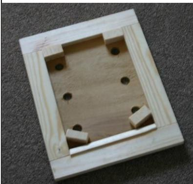
Build the door using lengths of wood and an oblong of plywood. Cut a series of ventilation holes in the plywood. Remember that another piece of plywood will make the inner skin for the door. This will have holes in different places to prevent a direct draught. This
