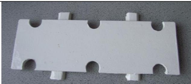
This was found to be the best method of making the inner skin of the bottom of the weather box. It simply rests in place. This means that it can be removed for cleaning. The two strips of wood lift the plate to create a ventilation slot.
