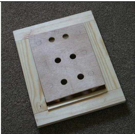
The inner skin is stuck onto the blocks of wood. The circles drawn onto this one show where the outer ventilation holes are. The photograph below shows the gap between the inner and outer layers.
