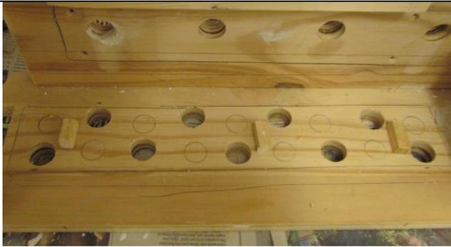
In order to make the side baffles removable for cleaning they were affixed using pegs and holes. A plastic peg set into a small block of wood (see right.) The strategy used here was to place the pegged blocks in place, then to stick the baffle to them and weight them down as they stuck. This made it possible to get the positions correct.
