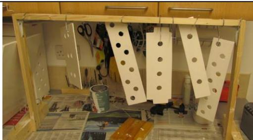
All parts were thoroughly painted. This included primer, undercoat and top coat. A drying rack was constructed to speed up this process.
