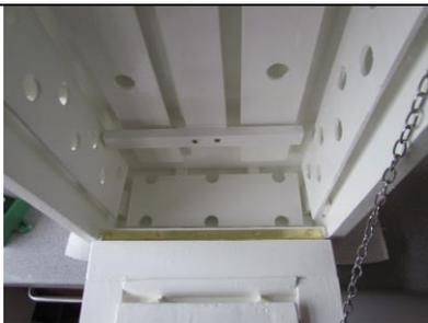
This is inside the finished weather box. Two cross pieces have been put on the back for hanging the thermometers on.
