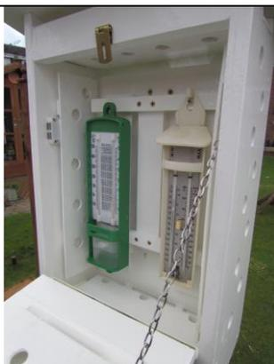
This shows how the thermometers are hung. The lower cross piece helps to keep the thermometers stable. This is especially useful when a button needs to be depressed to reset the thermometer.
